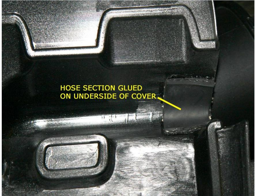
The result can be seen in the photo below. When the cover is installed, the hose section glued onto the underside of the cover cannot be seen. This solution allows the hose to be fully protected, but in a way that is not visible once the cover is installed.
