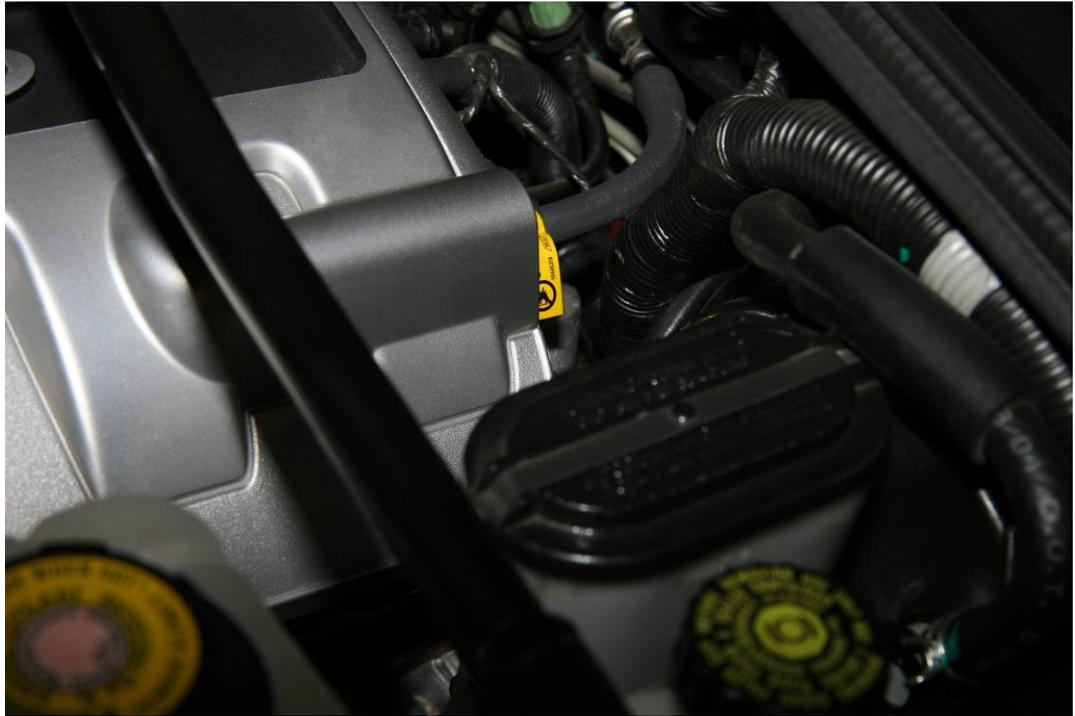
the fuel rail cover. Since one end of this line is fixed to the firewall and the other to the fuel rail, this line is constantly rubbing against the edge of the fuel rail cover as the engine shifts left and right during normal driving. Obviously, more aggressive driving causes even more relative motion and consequently more rubbing.
